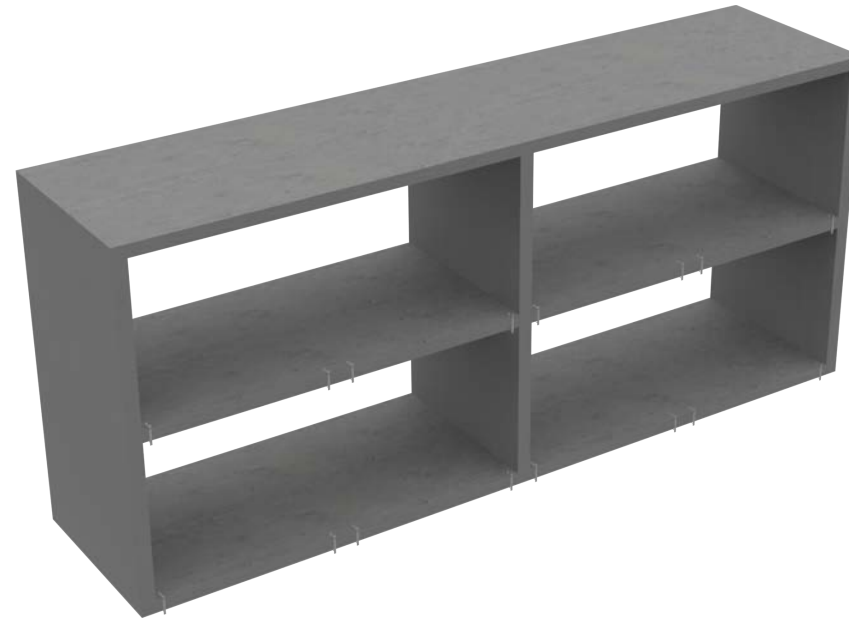
01b. Steel Anchors to support the prefabricated panels on the concrete slab.
