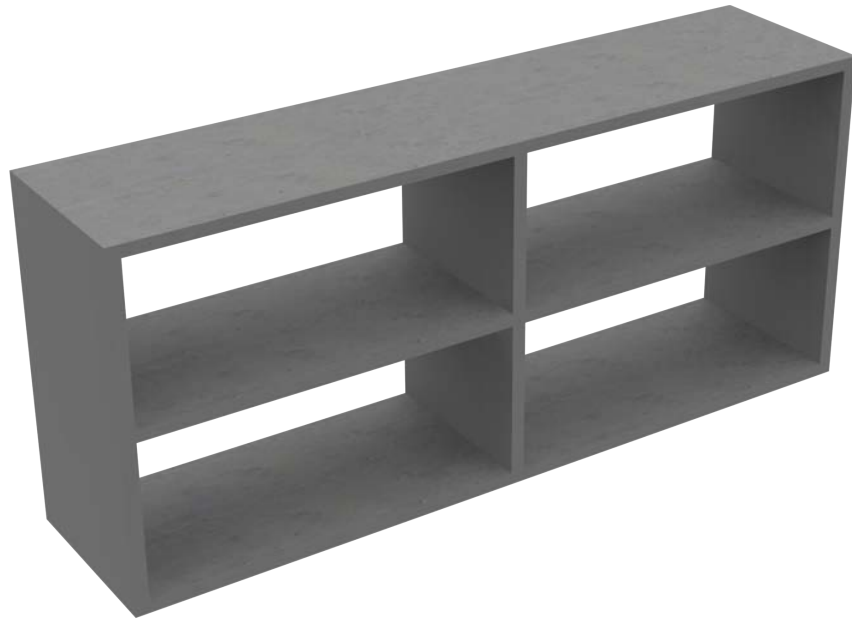
01a. Concrete Structure. Concrete walls cast on site. Concrete slab: 220 mm Concrete wall: 250 mm
